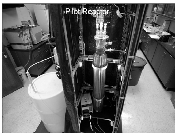
FIGURE 1 View of bioreactors with immobilized anammox bacteria used in this research. Left : upflow reactor with attached biomass. Right : scheme of the reactor with encapsulated biomass.
